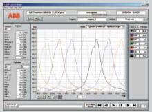
Deviations are continuously alarm monitored against performance references. The Cylmate Viewer is the first commercial tool on the market that has all information of the combustion process stroke-by-stroke, before the alarm, at the alarm, and after the alarm. That means it is possible to see the development of a fault and to get understanding of the mechanism that led to the fault.
