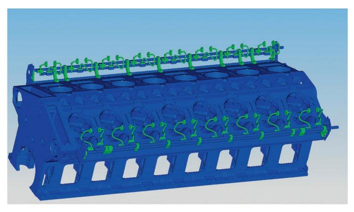
Improved support brackets for the main manifolds and S-shaped connecting pipes together help to prevent pipe cracks and fuel oil leakage.
