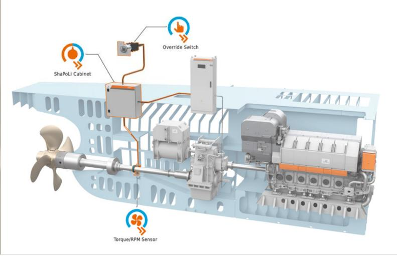
Wärtsilä Shaft Power Limitation is a complete upgrade package for vessels with Wärtsilä controllable pitch propellers. The fully integrated solution can be installed as an addon to Wärtsilä systems. System data is stored in accordance with the requirements of the ISO 19030 standard for performance monitoring. Wärtsilä Shaft Power Limitation has been designed in collaboration with one of the major classification societies to ensure a smooth approval process.
