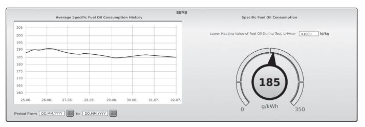
Example of Engine efficiency monitoring service user interface.
