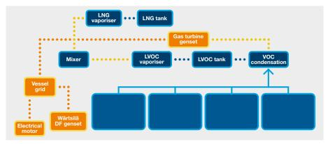
Emission transformed to fuel - 30-40% of fuel converted from waste
