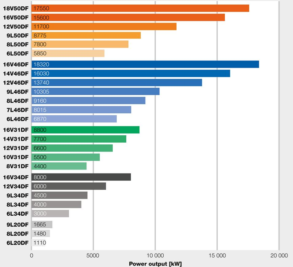
Wärtsilä's medium-speed dual-fuel engine portfolio for both main and auxiliary power production. The portfolio is available both for electrical and mechanical propulsion applications.
