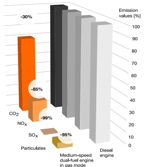
Example of emission reductions obtained by switching to gas.
