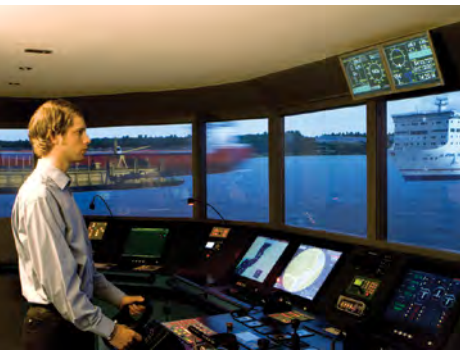
Interschalt AG, Germany. Integrated bridge systems supplied by Sperry, Raytheon and Transas are simulated
