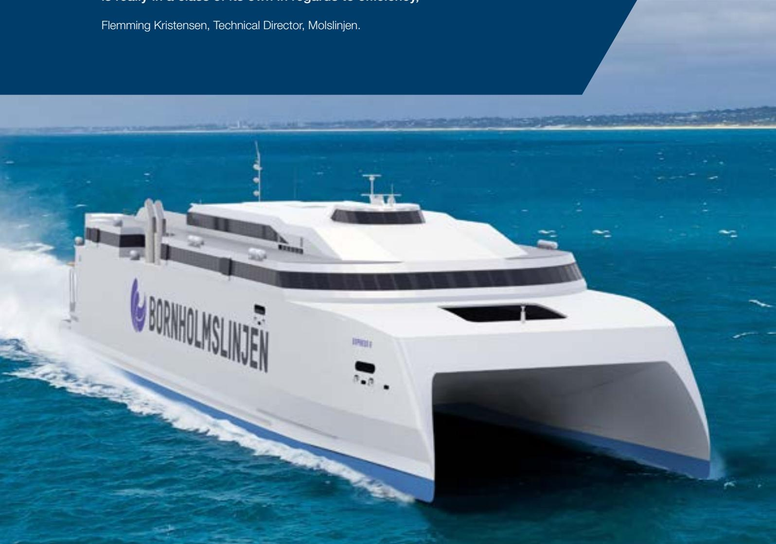
Integrated Wärtsilä 31 engines, WXJ1500SRI waterjets, and ProTouch powering the Express 5 Molslinjen high-speed ferry delivering optimised lifecycle reliability. Length 115 m.
