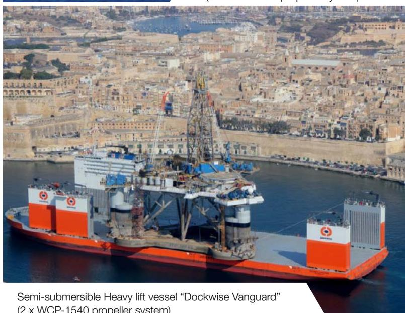
Semi-submersible Heavy lift vessel "Dockwise Vanguard"
