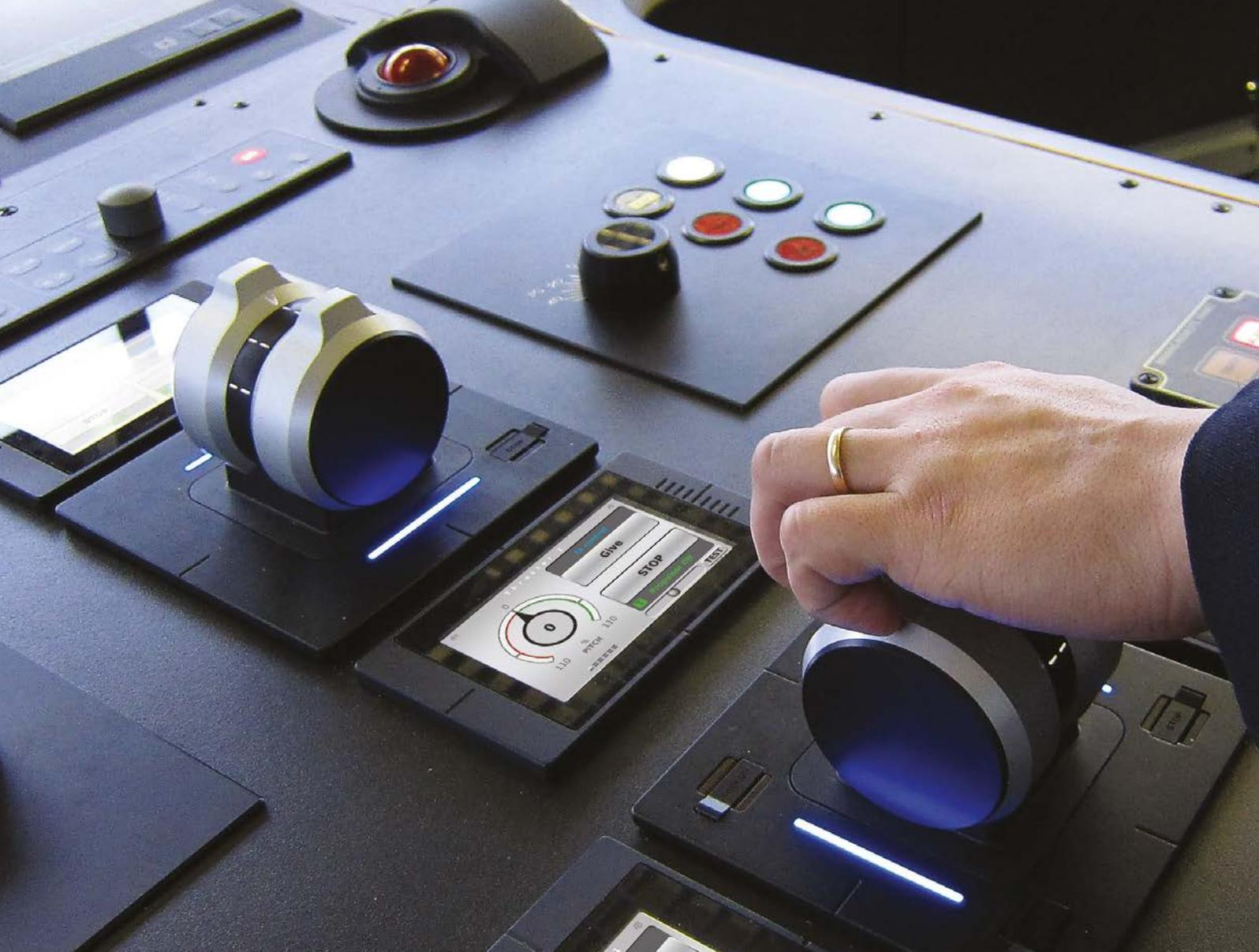
ProTouch, Wärtsilä's latest Propulsion Control System. Touch screen technology and solid ergonomics enable flexible bridge arrangements and intuitive control
