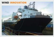
Wärtsilä has converted a Research/ Survey Vessel into a DP2 Walk-to-work Offshore Wind Support Vessel. The vessel has been upgraded with accommodation and hotel facilities for 125 people, and a heave compensated gangway. Our scope of supply was feasibility study, basic and detail design, yard specification, tender documentation and site supervision.
