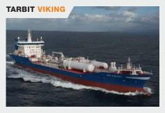
Designed by Wärtsilä Ship Design and built in 2007, Wärtsilä performed the entire conversion of the chemical tanker; the project consisted of the conversion of the diesel engines to dual-fuel; the installation of the entire LNG storage and handling system including the automation modifications. Tarbit Bit Viking is now sailing with very low NOx, CO<sub>2</sub> and zero SOx and PM emissions.
