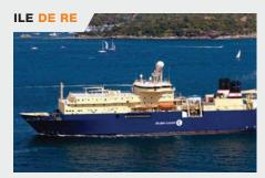
RO-RO vessel converted to cable layer, suitable to handle any type of underwater cable. Wärtsilä Ship Design ensured the feasibility of the concept and prepared the basic design and tender documentation package, including the yard specification.
