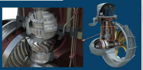
The spiral bevel gear-set, which is the heart of the thruster, has been thoroughly reviewed. Not only has the 8° gear angle been included in the gear geometry, the gear application and safety factors have been increased and a high quality gear material has been selected.
