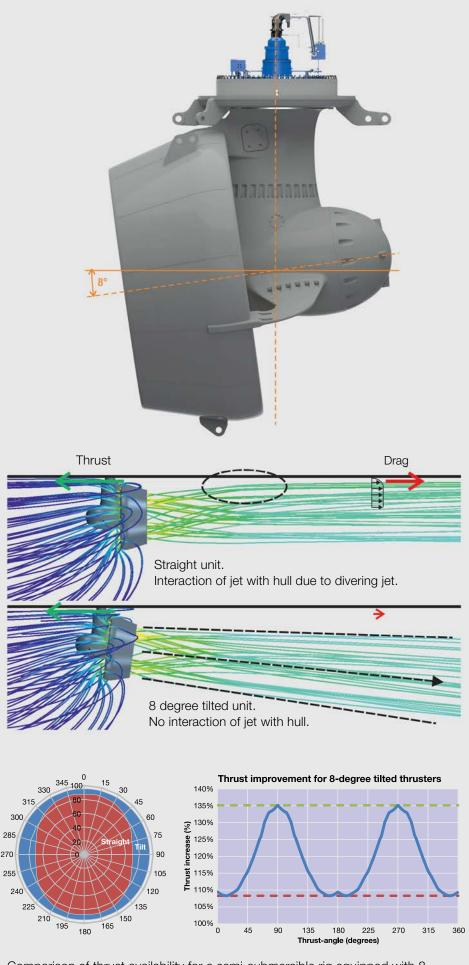
Comparison of thrust availability for a semi-submersible rig equipped with 8 thrusters. The red area shows the thrust availability in case of non-tilted thrusters, the blue area shows the available thrust in case of Wärtsilä Steerable Thrusters with an 8 degree downward tilt. Depending on the angle in which the thrust is directed, up to 35% more thrust is available for the rig equipped with the 8 degree tilted thrusters.
