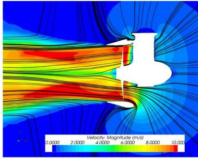
Wärtsilä Thruster Nozzle (WTN) optimised for bollard pull
