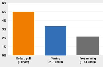
Performance improvement with the HP nozzle compared to 19A nozzle for a typical 150 ton AHTS.
