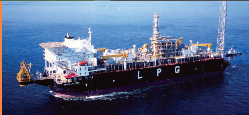
Wärtsilä LPG reliquefaction plant onboard 135,000m 3 LPG FPSO Sahnä
