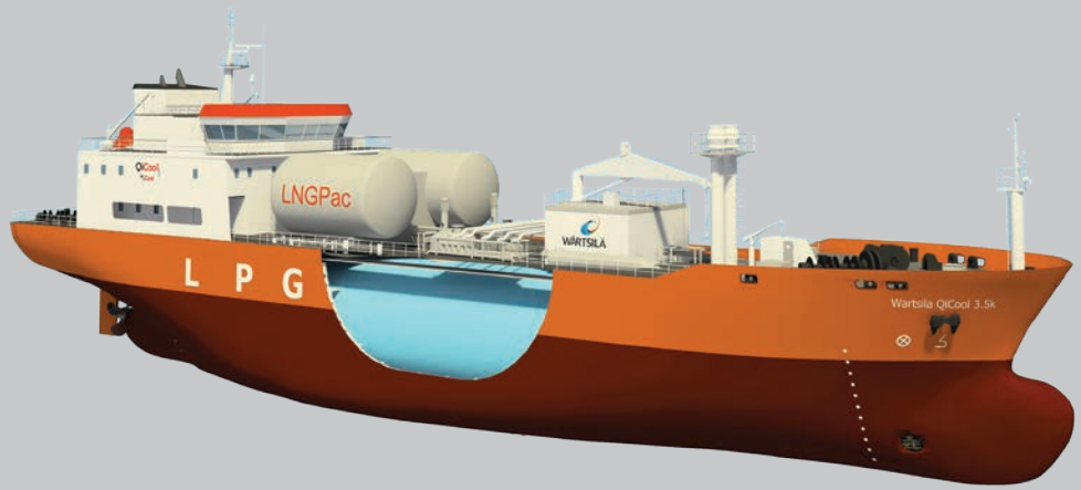
3,500m³ LPG carrier of new QICool type
