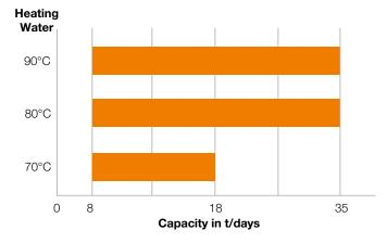
Capacity based on 32° C seawater
