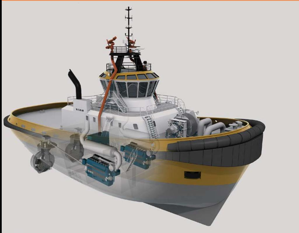
in the mid of 1990s. Wärtsilä 34DF covers the middle part of the power range in the dual-fuel Wärtsilä engine family. Available cylinder configurations are 6, 8 and 9 in-line, and 12 and 16 Vee- configurations covering the power range from 2.8 MW to 8.0 MW. Speed range is 720–750 rpm for use with 50 or 60 Hz applications.
