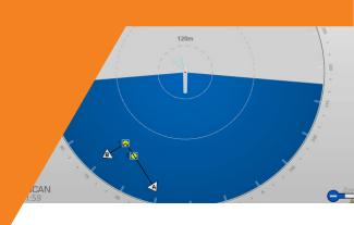
RadaScan provided by Guidance Marine is an advanced premium position reference sensor for long range use in marine Dynamic Positioning (DP) applications.
