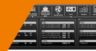
The Wärtsilä Fleet Pilot System allows the collection of data on a ship's substation, which can then be synchronized on a shore based server. The data received are logged and displayed at the remote station located in the customer's offices. The system enables signals received from different vessels of the fleet to be monitored and stored at the same time.
