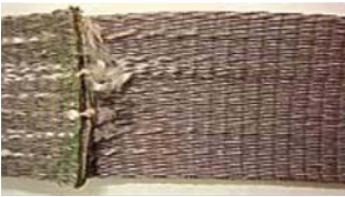
The sling stitching is ripped.
