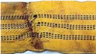
The cut or friction damage exceeds 10% of the sling width.
