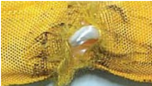
Core of the round sling is exposed.
