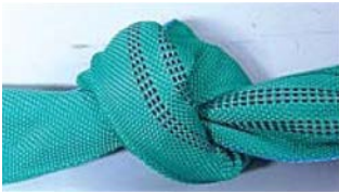
There is a knot in the webbing sling/round sling.
