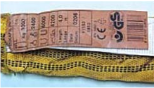
Working load markings are illegible.
