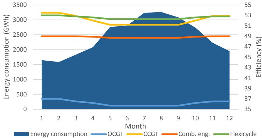
Figure 12: Monthly expected average efficiency in Abu Dhabi and monthly energy consumption
