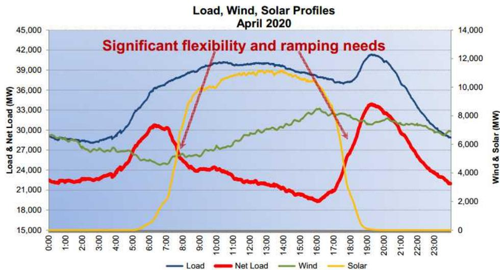
Figure 1: Flexibility is paramount to deal with future grid dynamics in California (Skinner, 2012)
