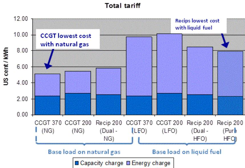
Figure 5: At 66% PLF and full load, CCGT offers better performance
