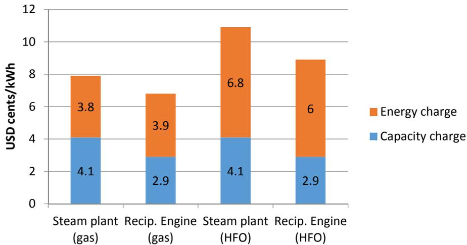
Figure 7: Tariff comparison for flexible loading
