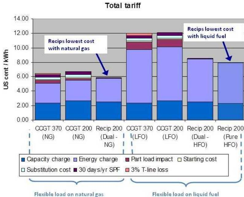
Figure 6: However, for flexible load operations, reciprocating engines offer clearly the best performance
