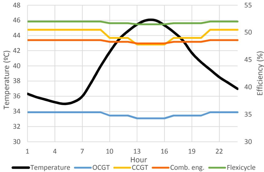
Figure 14: Hot day efficiency impact of the different generation technologies
