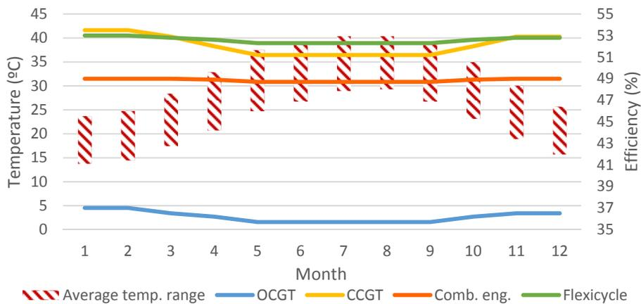
Figure 11: Monthly expected average efficiency in Abu Dhabi, depending on temperature range
