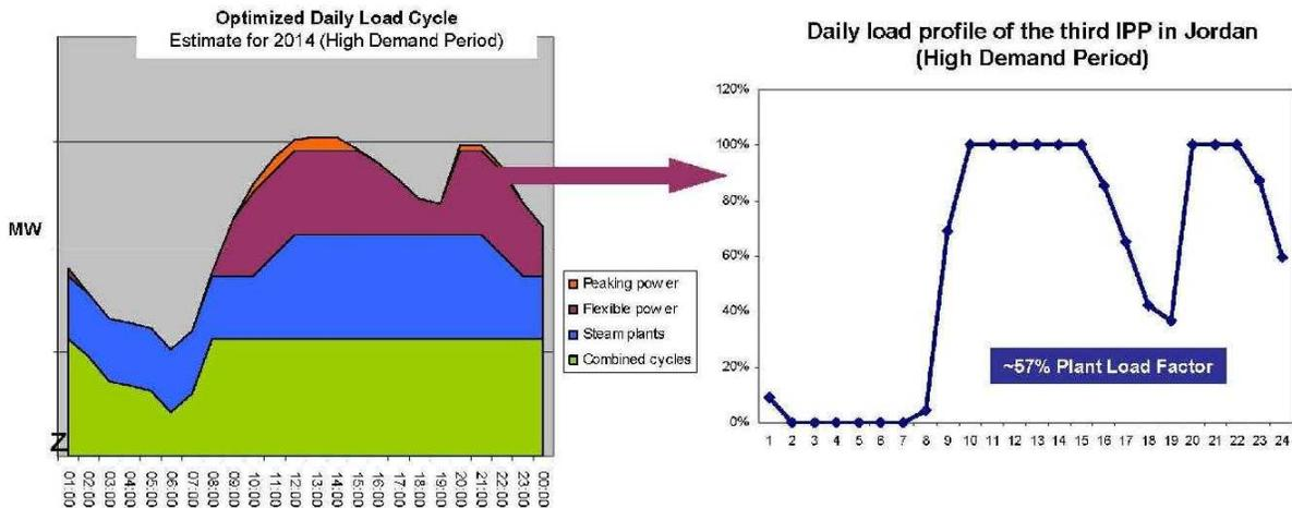
Figure 4: Daily load profile of proposed third IPP plant in Jordan. Please note how the Smart Power Generation capacity (purple) absorbs the peaks and allows the existing CCGT capacity to run at full load and full efficiency (M. Al Azzam & Paldanius, 2014)
