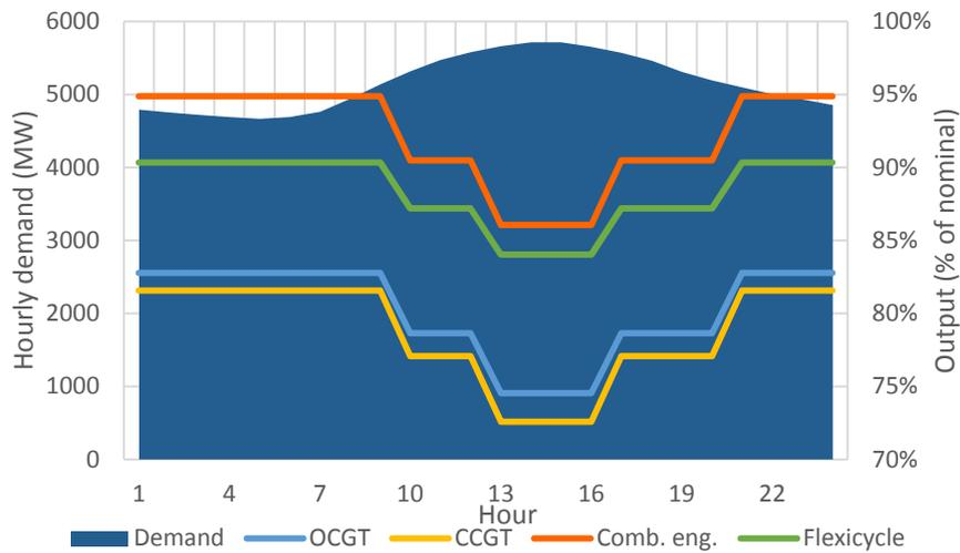
Figure 15: Hot day de-rating of the different generation technologies
