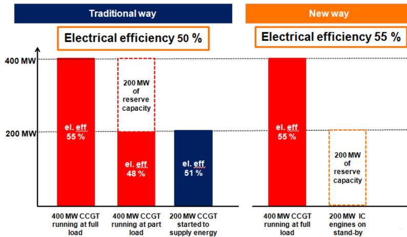
Figure 16: Power system optimisation with non-spinning reserves (Hultholm, 2014)
