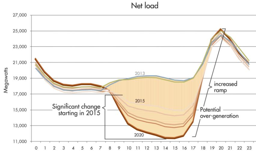
Figure 2: Development of the net load in California, 2013 – 2020 (Rothleder, 2013)
