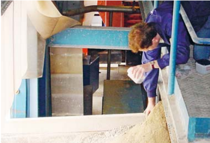
■ Fig. 1 – Gathering end product samples for later analysis from a diesel power plant equipped with flue gas desulphurization (FGD) .
