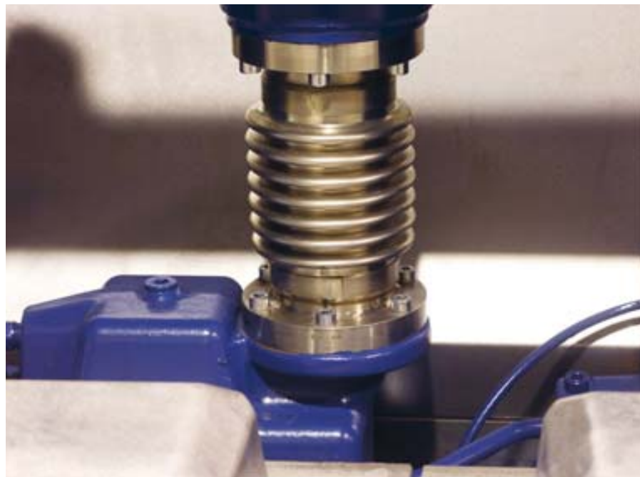
■ Fig. 5 – Gas admission valves for supplying gas to the cylinder.
