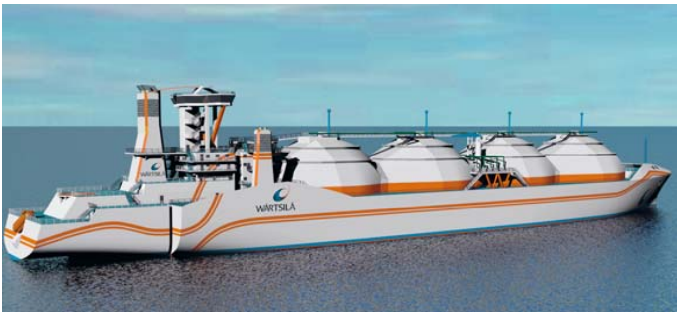
■ Fig. 1 – Artist impression of the open water tug pushing the LNG barge in open water.
