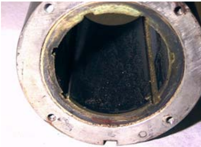
■ Fig. 8 – Ecosafe bearing and shaft after test.
