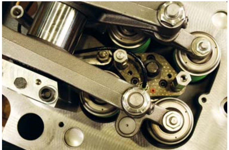
■ Fig. 4 – Twin-needle injection valve with electronically operated pilot injection.
