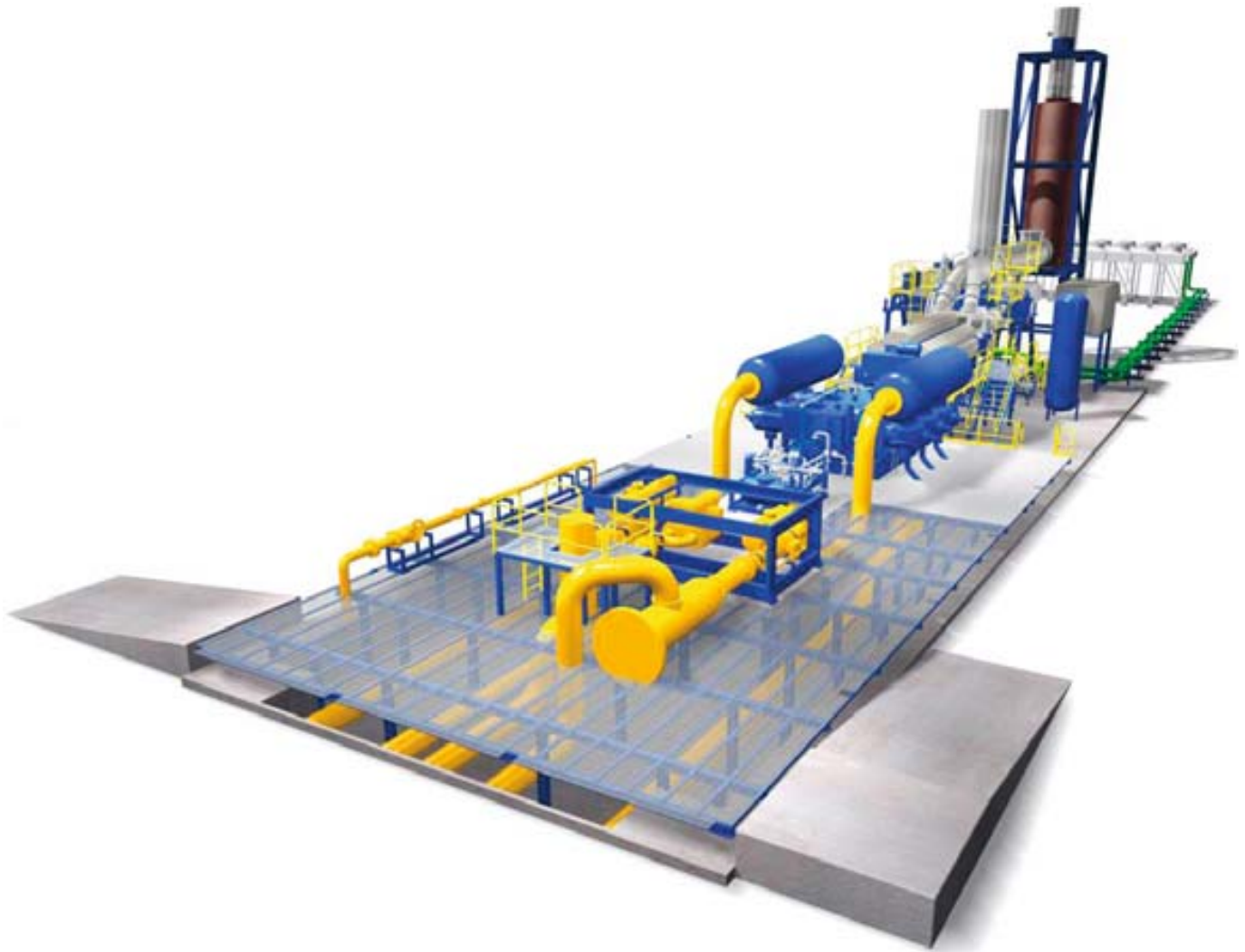
■ Fig. 4 – Wärtsilä engine powered compression equipment.
