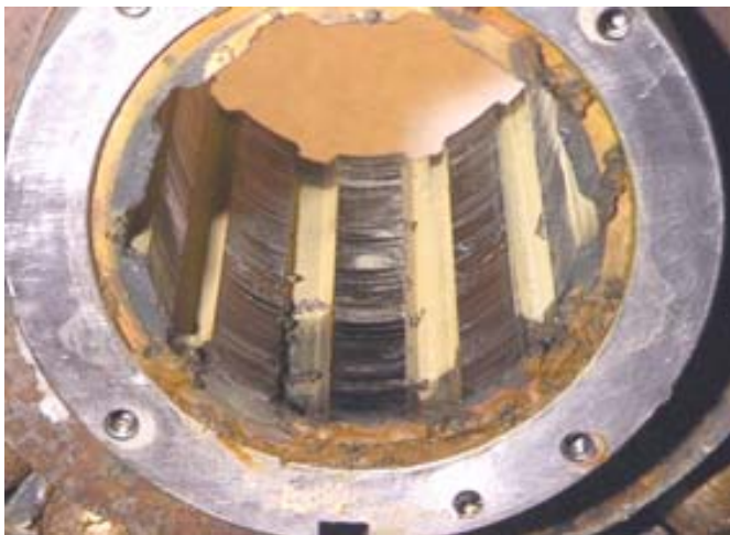
■ Fig. 6 – Rubber bearing and shaft after the test.
