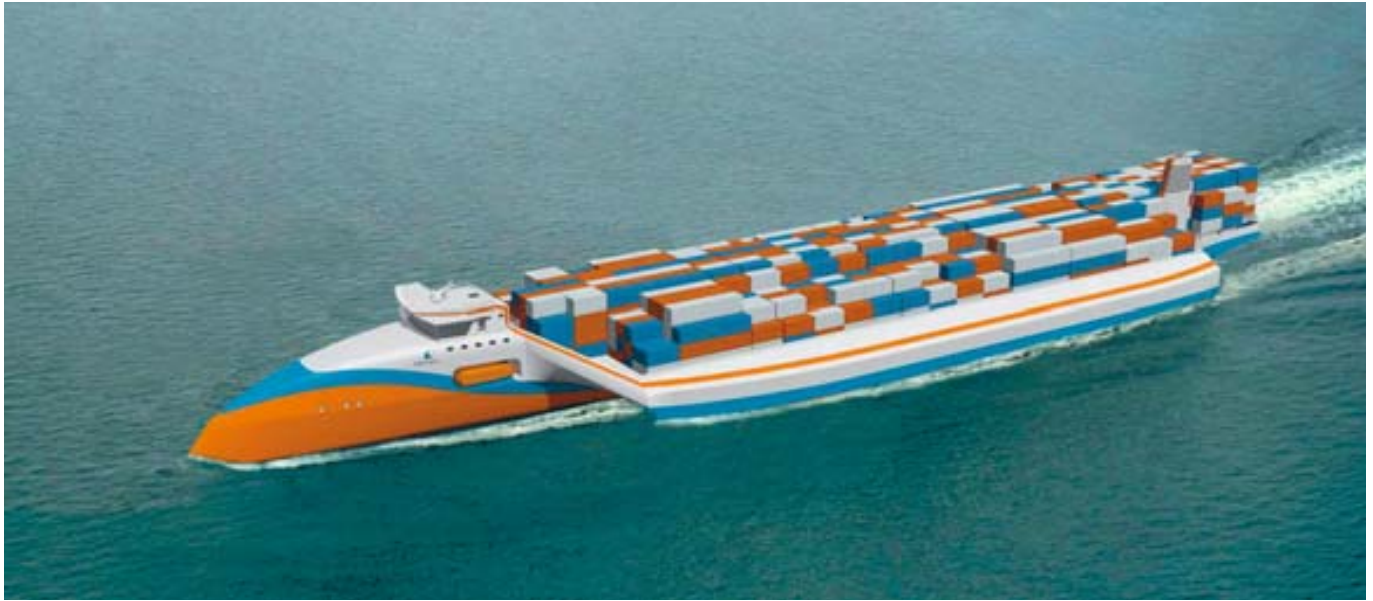
■ Fig. 1 – The novel container feeder concept featuring a long slender hull with an outrigger on the port side.
