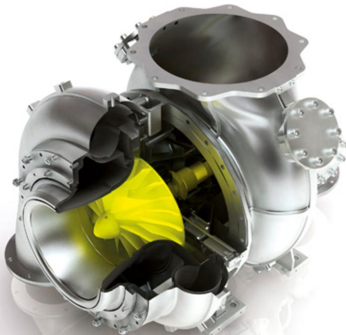
The Napier 307L features a wider compressor map, which enables greater operational flexibility by increasing the turbocharger's speed margin. In addition, thermal stress is reduced because of the lower turbine inlet temperature. The level of SFOC reduction enabled by the upgrade depends on installation and site conditions, but the approximate savings can be as much as 3%.
