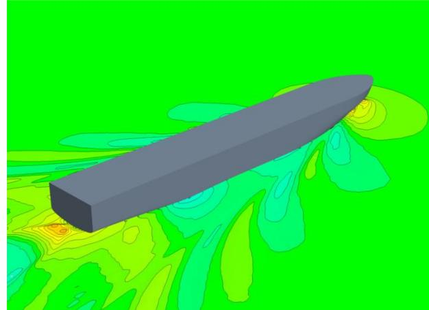
Figure 5: Pressure distribution and wave profile.
