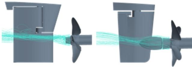
Figure 6: Conventional rudder vs. Energopac.
