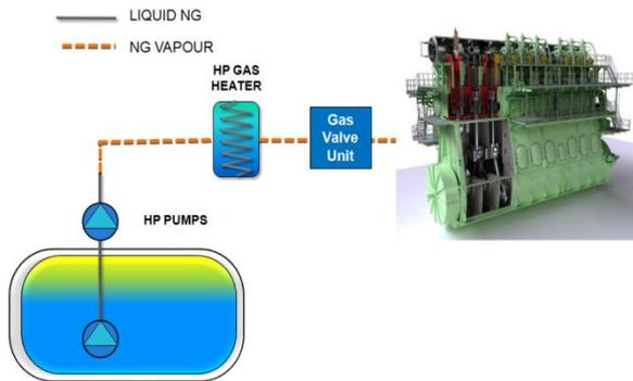
Figure 8: Main engine MAN & TGE HP FGSS
