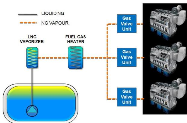
Figure 9: Auxiliary engines MAN/TGE LP FGSS
