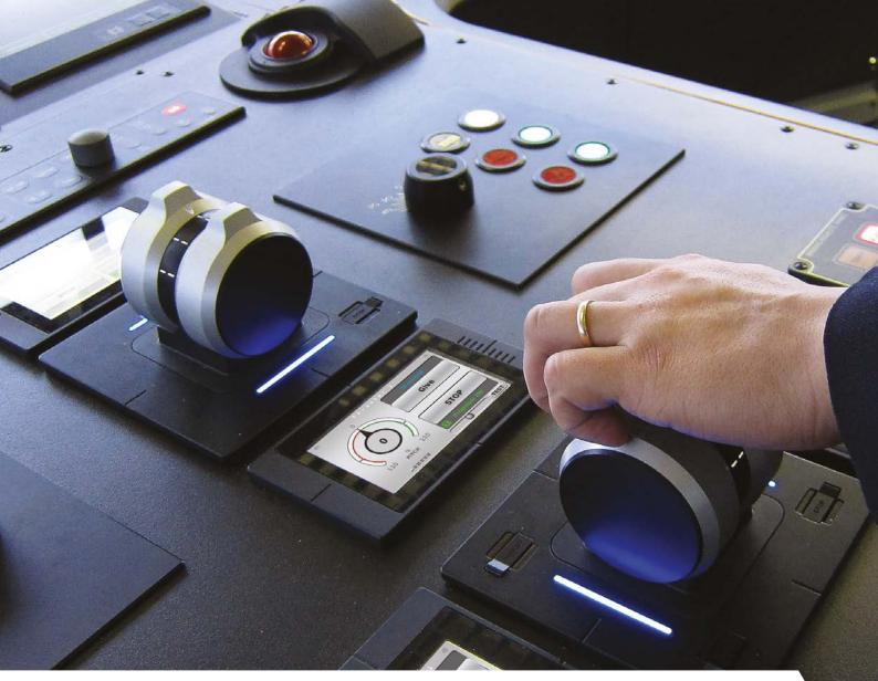
ProTouch, Wärtsilä's latest Propulsion Control System. Touch screen technology and solid ergonomics enable flexible bridge arrangements and intuitive control
