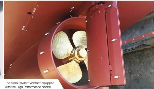
with the High Performance Nozzle (1 x WCP-1000 propeller system)
