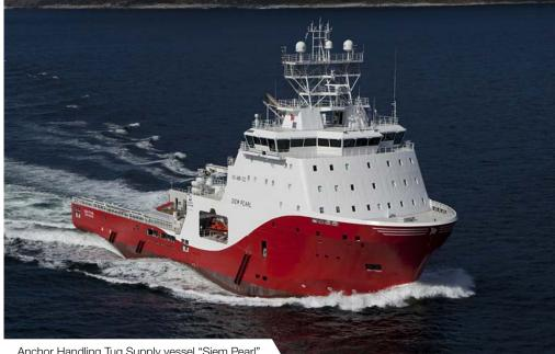
Anchor Handling Tug Supply vessel "Siem Pearl" (2 x WCP-1190 propeller system)
