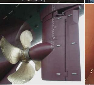
The multi-purpose vessel "Dynamogracht" equipped with the fuel efficient Energopac system. (1  $\times$  WCP-1540 propeller system)
