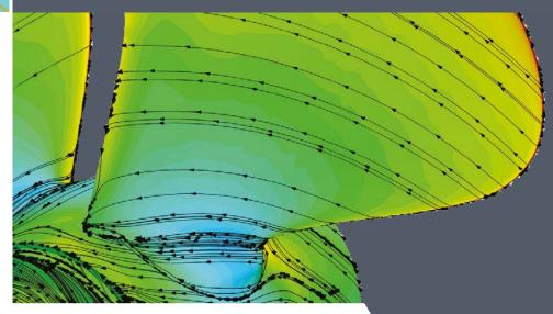
Detailed state-of-the-art Computational Fluid Dynamic analysis of the hub and blade design hydrodynamics
