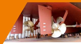
The Wärtsilä Controllable Pitch propeller systems have been developed to provide outstanding reliability, low operating costs, environmental friendliness, easy installation/integration, and intuitive operating control. Wärtsilä designs and produces controllable pitch propellers for the commercial, navy and superyacht markets. It is a unique product from which the first design dates back to 1903. Today Wärtsilä has accumulated a wealth of experience with more than 20,000 units installed.
