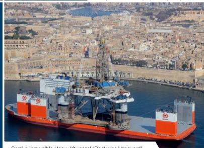
Semi-submersible Heavy lift vessel "Dockwise Vanguard" (2 x WCP-1540 propeller system)
