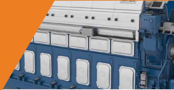
The Wärtsilä 46DF is a four-stroke dual-fuel engine that can be run on natural gas, heavy fuel oil (HFO) or marine diesel oil (MDO). The engine can smoothly switch from gas fuel to HFO/MDO operation and vice versa without loss of power or speed. The Wärtsilä 46DF design is based on the well proven and reliable Wärtsilä 46F and Wärtsilä 50DF engine families, which have operated successfully on the market since the early 2000s.
