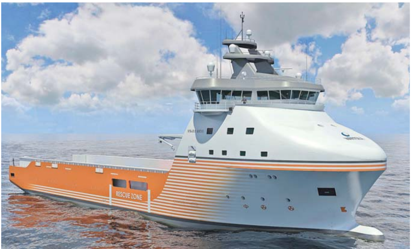
■ Fig. 1 - The Wärtsilä VS PSV 485 MKIII design platform supply vessel features the Wärtsilä Low Loss Concept solution.
