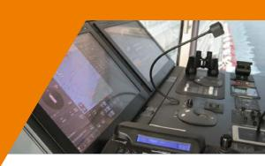
The Joystick System has been designed to provide easy control of vessel movement. The product consists of 2 modules – an Operator Workstation including a 3 axis non-spring loaded joystick, and a Signal Processing Unit (SPU). Connection to the thrusters is simplified through the use of I/O modules within the SPU. The product can be upgraded to DPO with the addition of an MRU and a DGPS; and to a DP1 with the addition of a second SPU and Operator Workstation.
