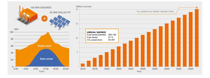
**Figure 8** Assuming delivery price of 50 USD/barrel, the fuel cost savings are 10 million USD per year. In carbon emissions, the reduction is equally 21 percent, or approximately 83 000 tonnes per year.
