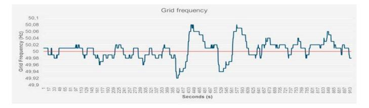
Figure 9 Grid Frequency Control with Energy Storage.
