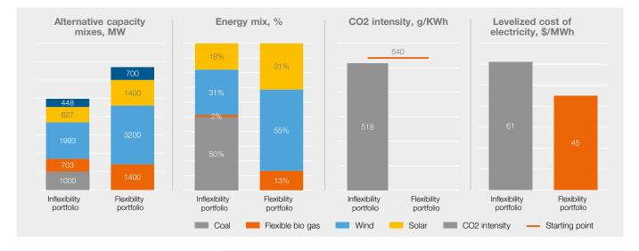
Figure 7 Comparing two alternative scenarios in an energy system with good wind and solar conditions for PNM New Mexico.
