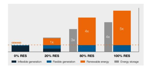
Figure 5 Capacity vs peak demand models for a 100% RES show a massive investment in renewable generation capacity is required.
