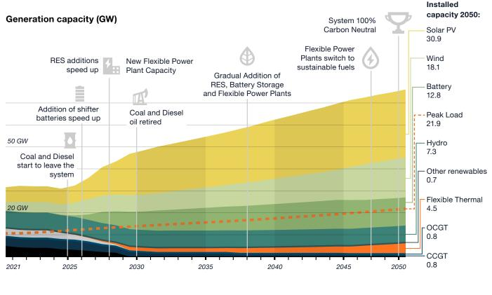
● Coal ● CCGT ● OCGT ● Diesel ● Flexible Thermal ● Other Renewables ● Hydro ● Battery ● Wind ● Solar PV ···· Peak Load ···· Electricity Demand
