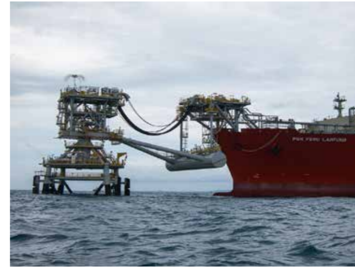
■ Fig. 15 - PGN FSRU Lampung, where Wärtsilä has delivered 3 regasification trains with max capacity of 360 TPH. Photo: Höegh LNG.
