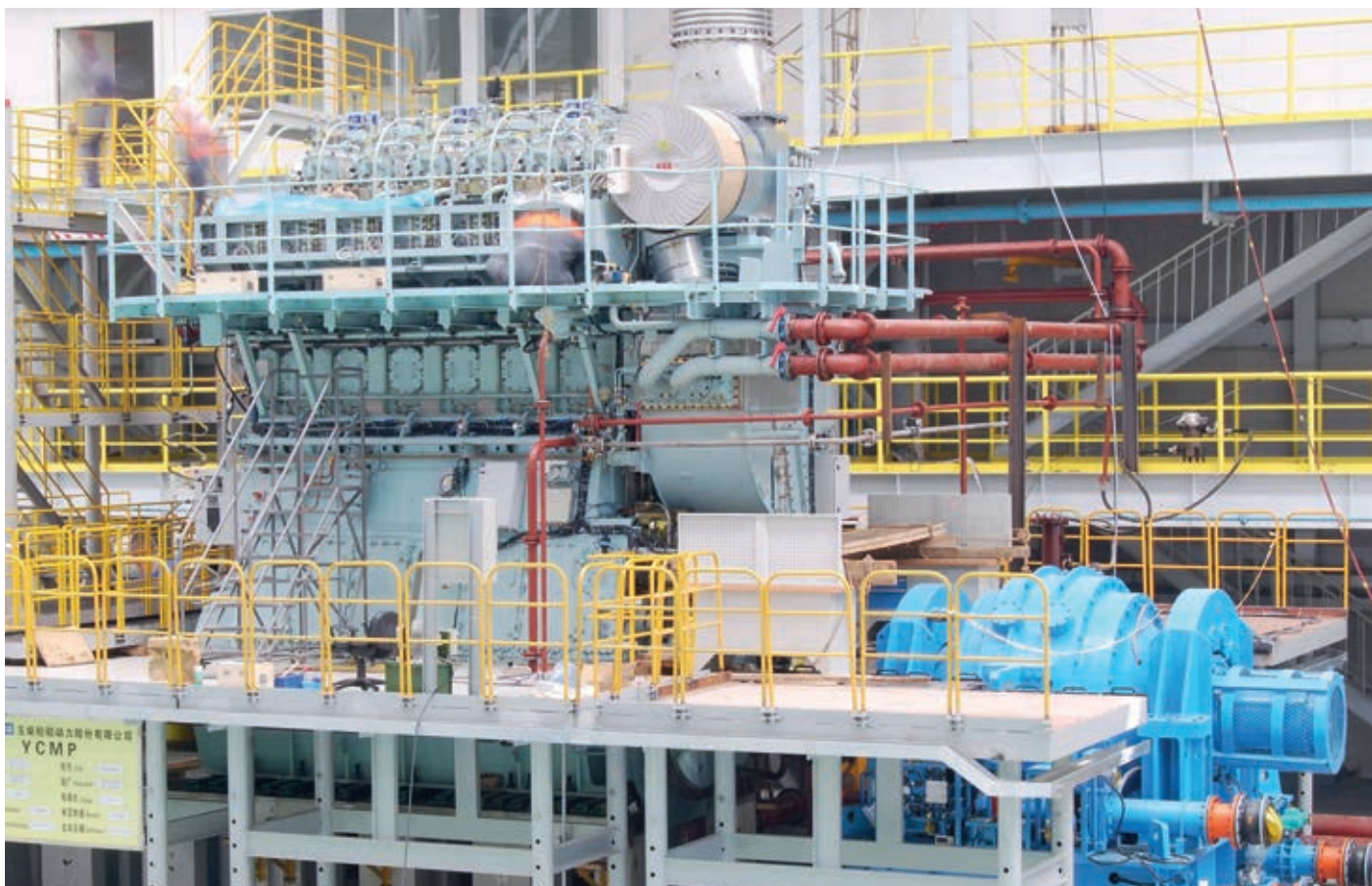
The Wärtsilä X35 engine is a two-stroke, slow speed diesel engine.
