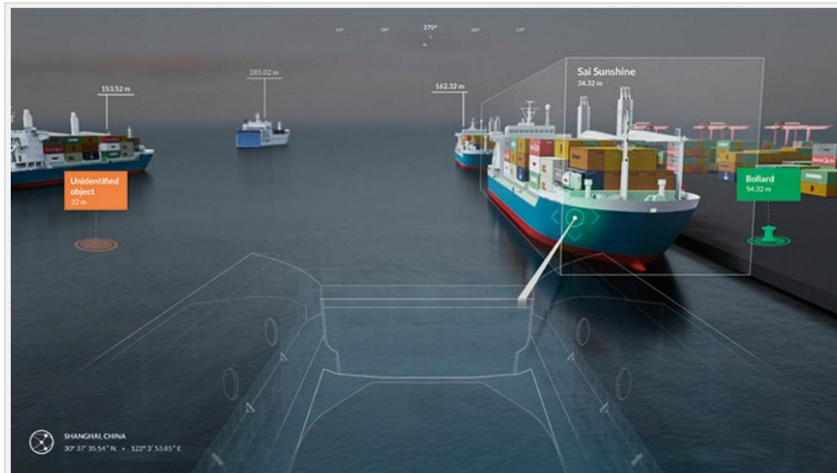
Rolls-Royce Intelligent Awareness Navigation System (pictured) uses sensors to give seafarers a 3D model of nearby vessels and hazards. Credit: Rolls-Royce
