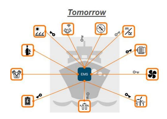
The performance focussed energy management system (EMS) is a new software category on a vessel and sits on top of the safety focussed Power Mmgt. System (PMS)
