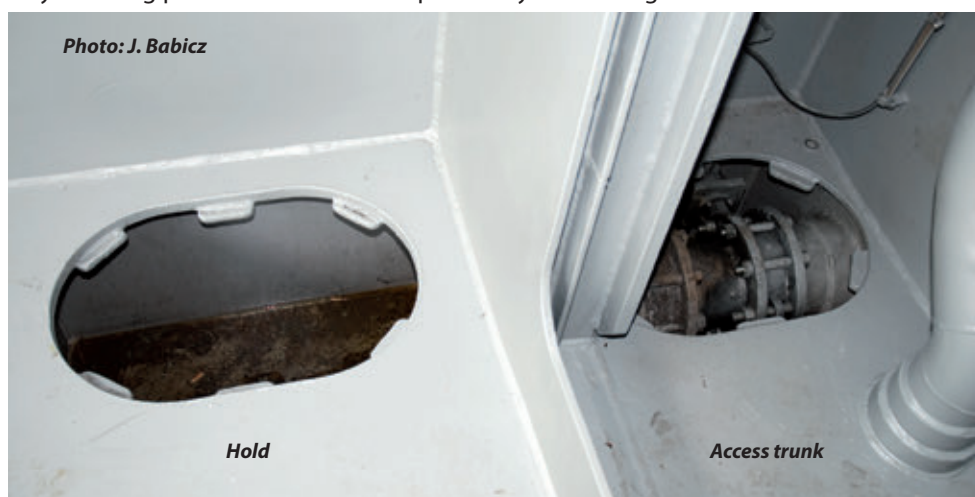
Always accessible bilge well designed by BNC
