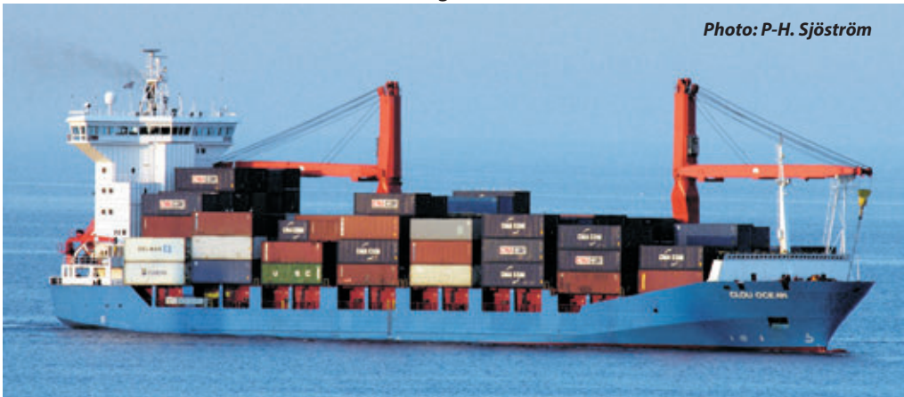
Feeder vessel: note the enclosed bridge
