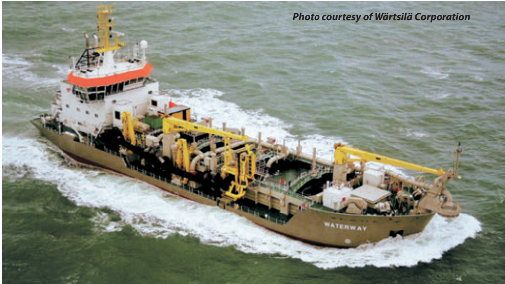
Trailing suction hopper dredger WATERWAY
