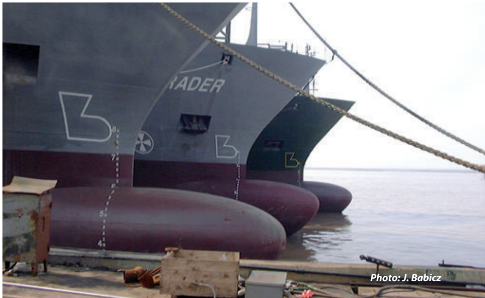
Long and strong bulbs can be perfect tools to sink rammed ship
