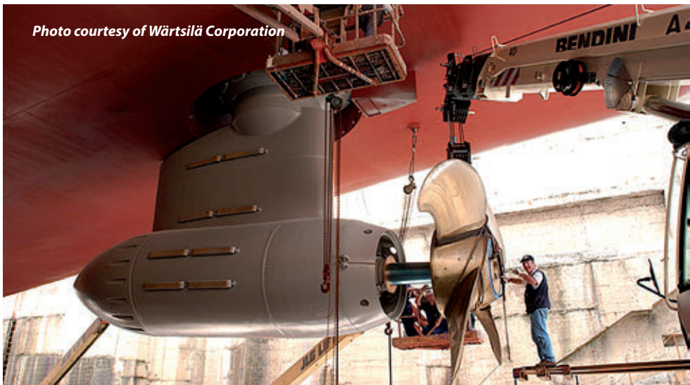
Podded propulsor DOLPHIN developed by Wärtsilä Lips and German electronic company STN ATLAS
