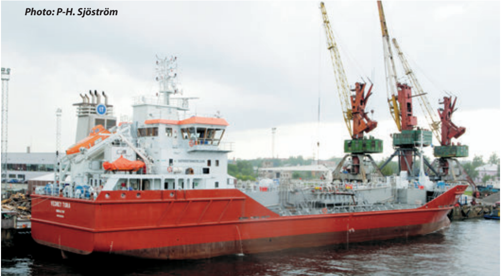
3515dwt product carrier VEDREY TORA LBP = 75.00m, Bmld = 15.70m, Dmld = 7.80m
