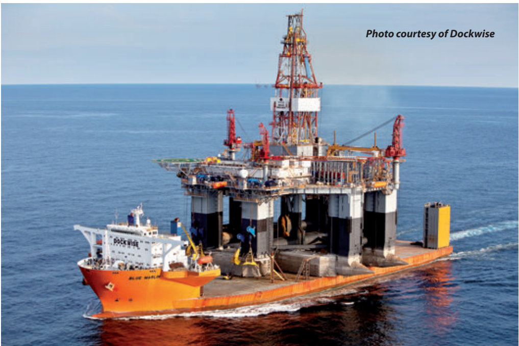
Semi-submersible heavy-lift vessel BLU MARLIN
