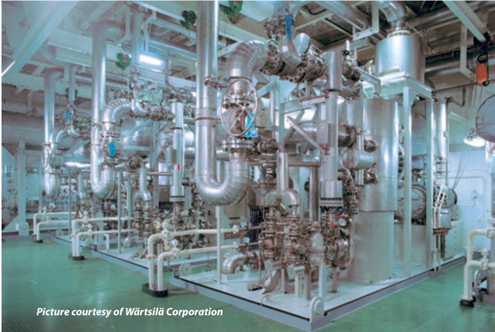
Reliquefaction plant onboard SANHA LPG FPSO
