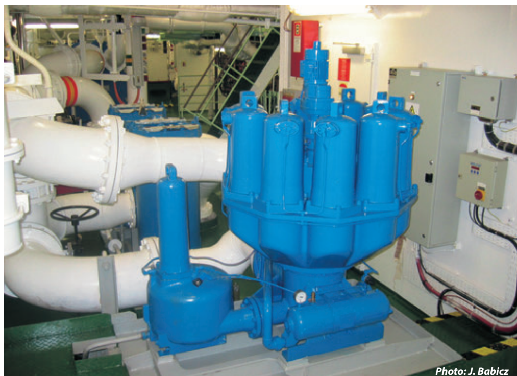
BOLL&KIRCH automatic lub. oil filter with flushing liquid treatment unit
