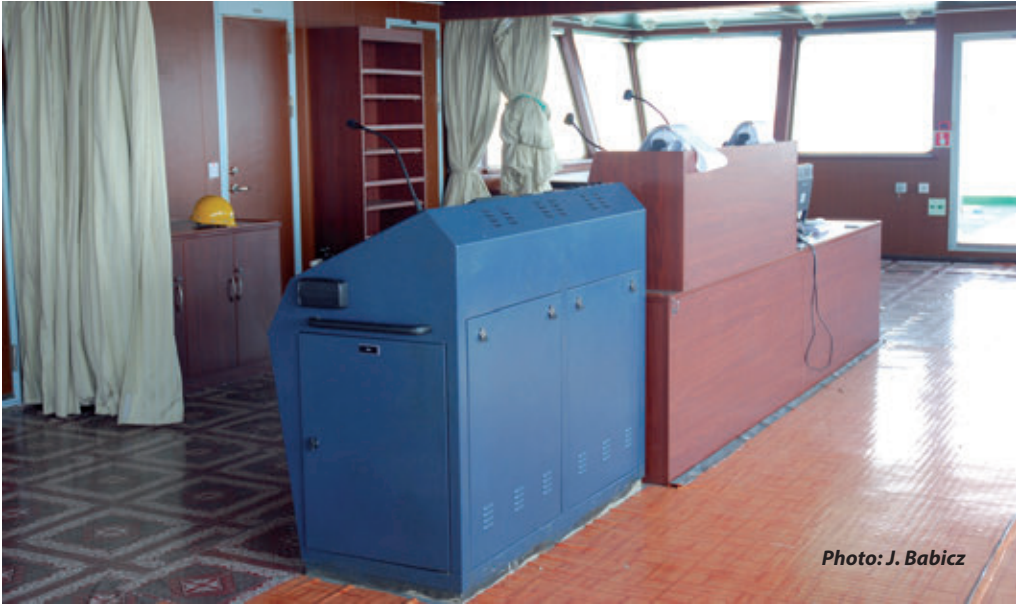
Wrong wheelhouse arrangement with high equipment located in field of vision
