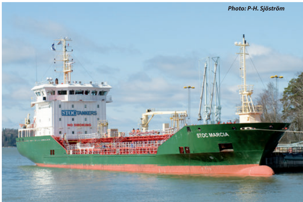
4634dwt oil/chemical tanker STOC MARCIA L_{BP} = 94.04\text{m} , B_{mld} = 15.00\text{m} , D_{mld} = 7.40\text{m} , d = 6.00\text{m}
