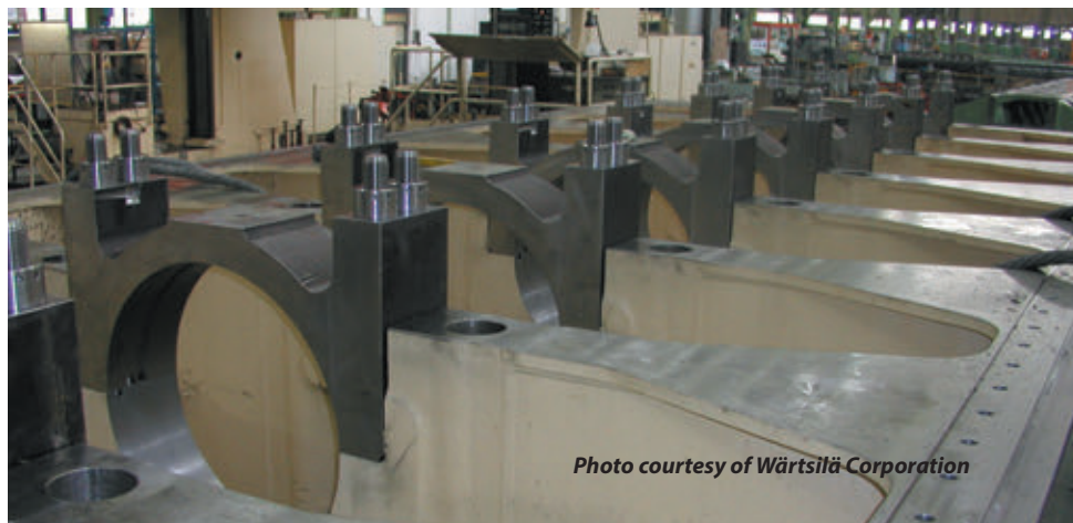
Bedplate of the 7RT-flex60C engine with main bearing caps in place
