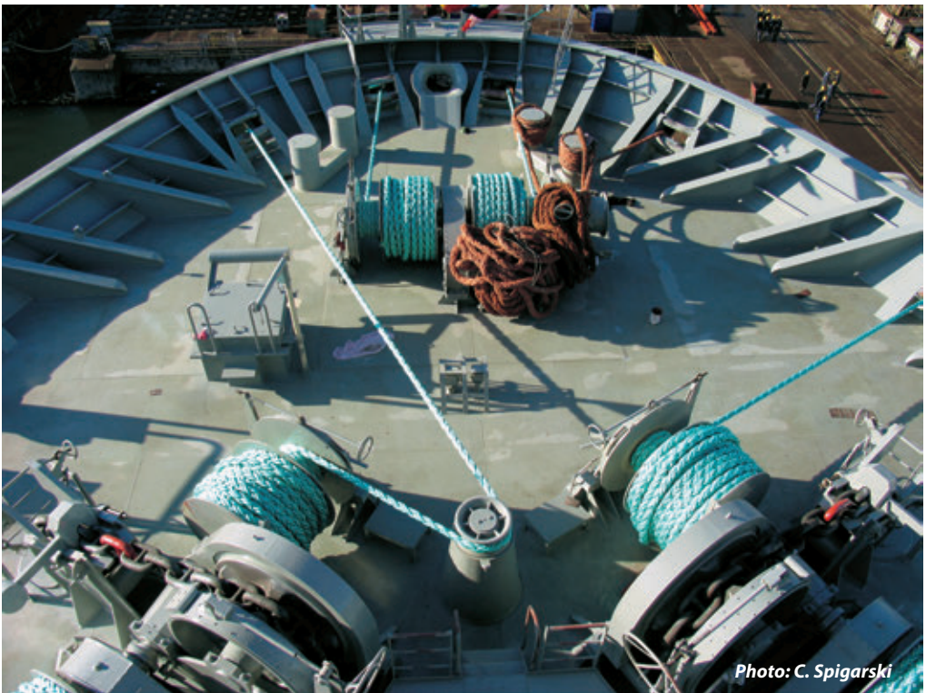
Anchor/mooring equipment on the forecastle deck of 4444 TEU vessel
