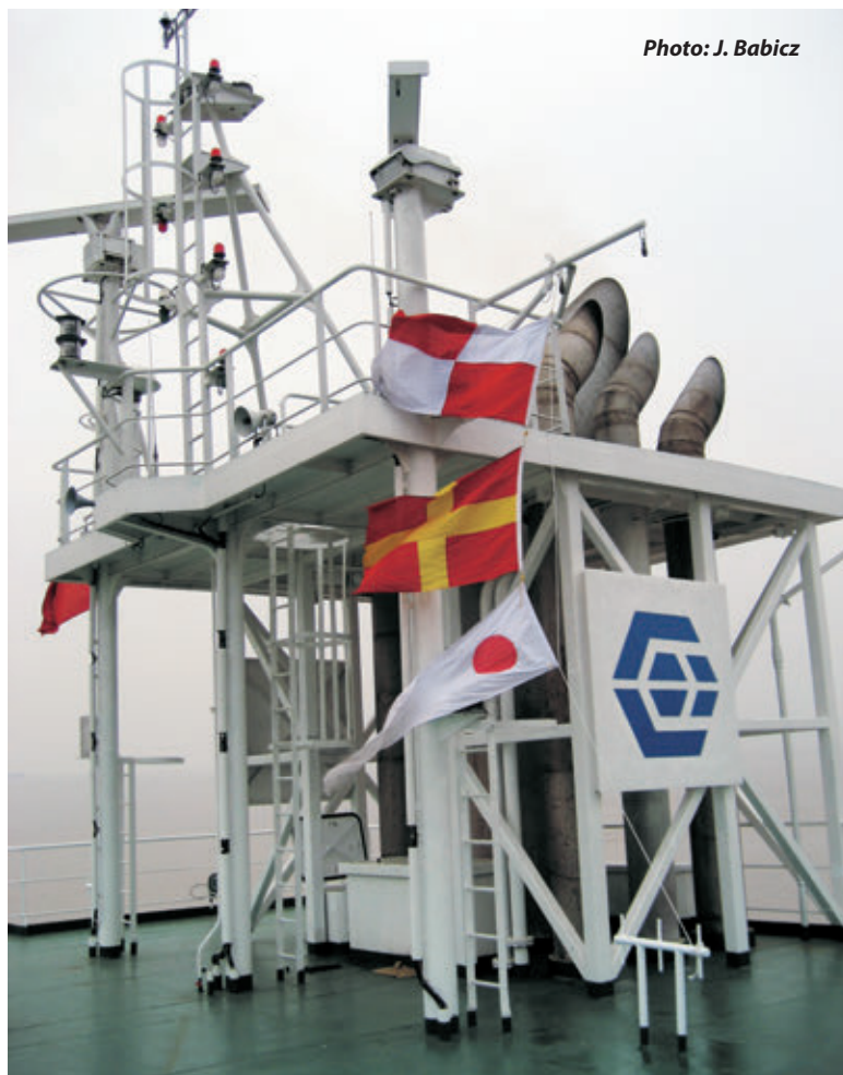
Unconventional funnel connected with signal and radar masts
