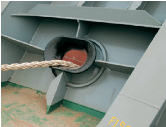
Chocks can be bulwark- or deck mounted
