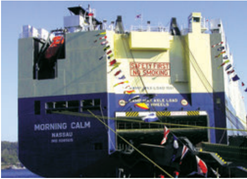
Free-fall lifeboat and launching ramp with integral recovery system onboard car carrier
