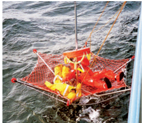
Rescue lifting system with double loop and stopper block
