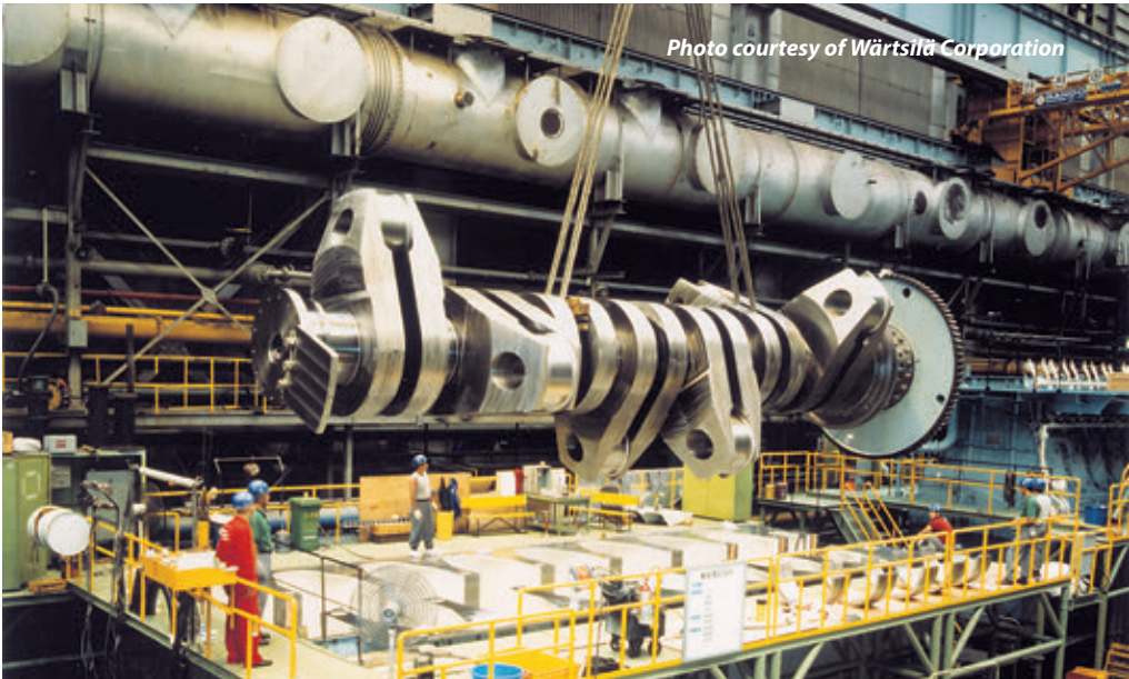
Fitting the crankshaft into the bedplate
