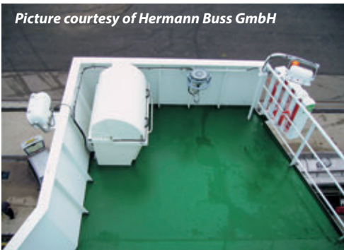
Wrong wheelhouse arrangement with high equipment located in field of vision
