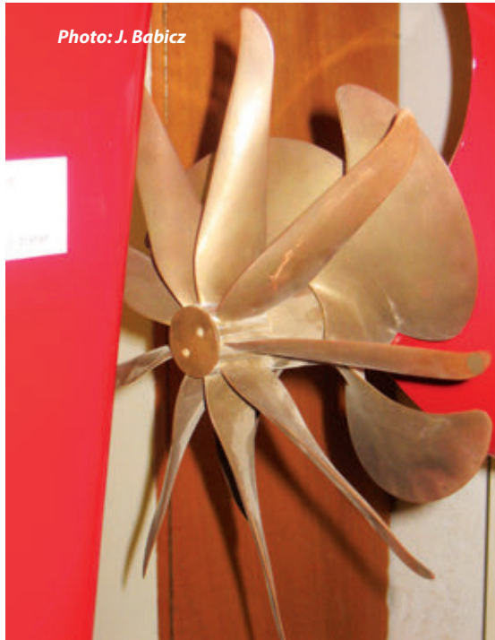
The model of Grim vane wheel at Hamburg Ship Model Basin
