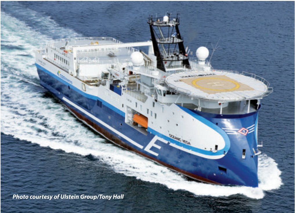
X-Bow Seismic Research Vessel OCEANIC VEGA
