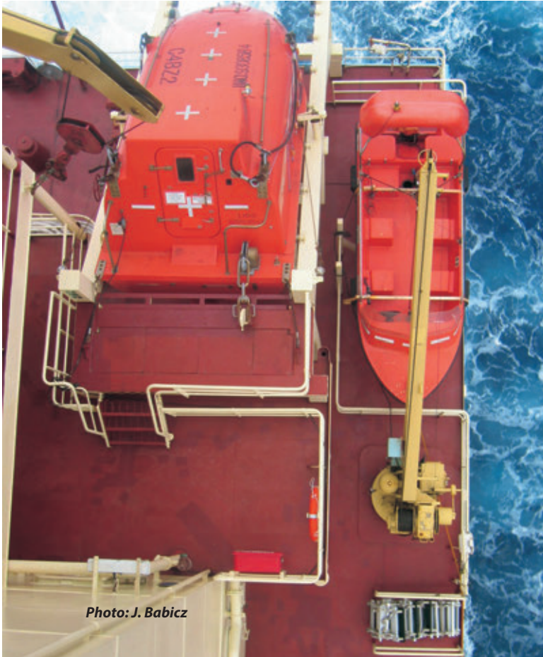
Launching arrangement for free-fall lifeboat, rescue boat and 25-person liferaft
