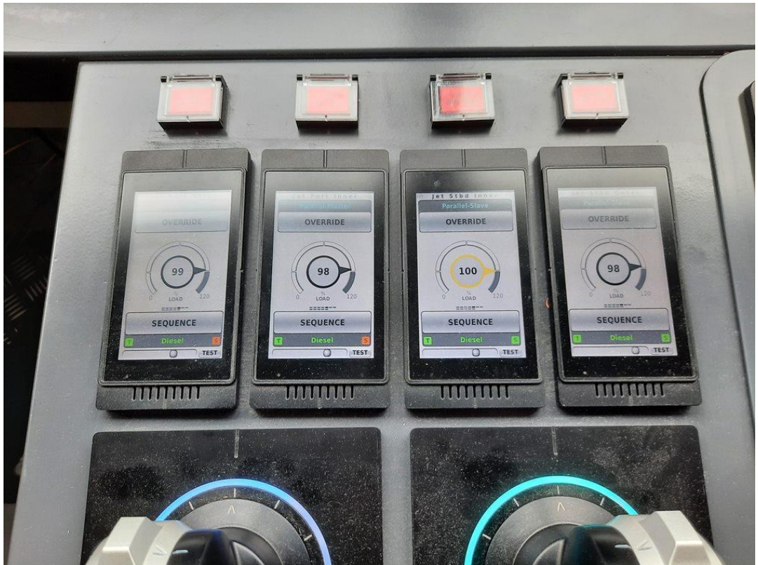
Image 2: ProTouch waterjets control for the 4 jets
