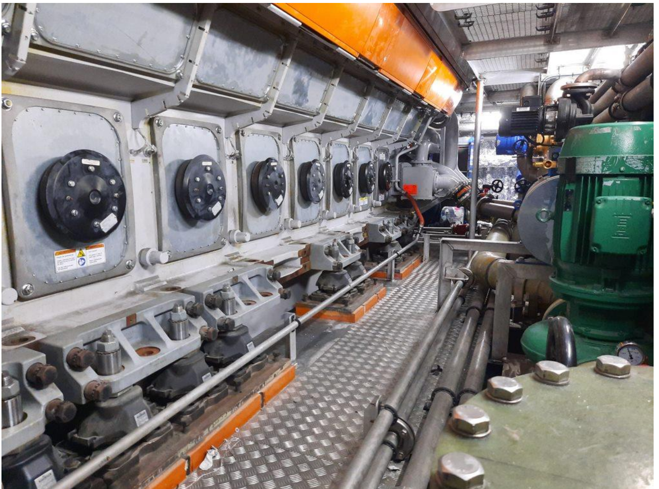
Image 11: Lower engine room W31DF crank case cover
