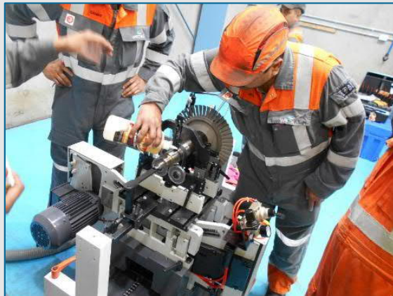
Balancing rotor shaft
