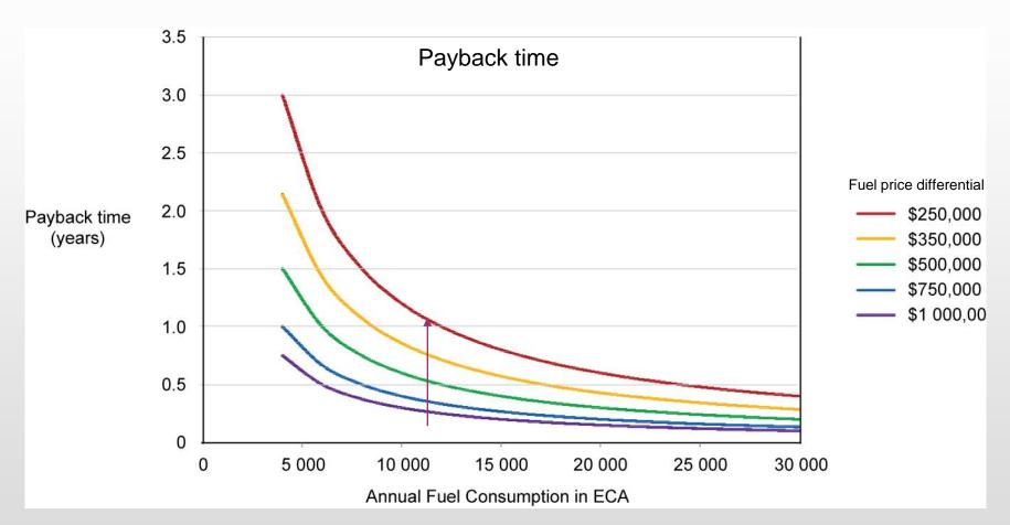
10 MW Main Engine, 3x0,5MW Aux. Engines, Total investment cost USD 3.000.000
