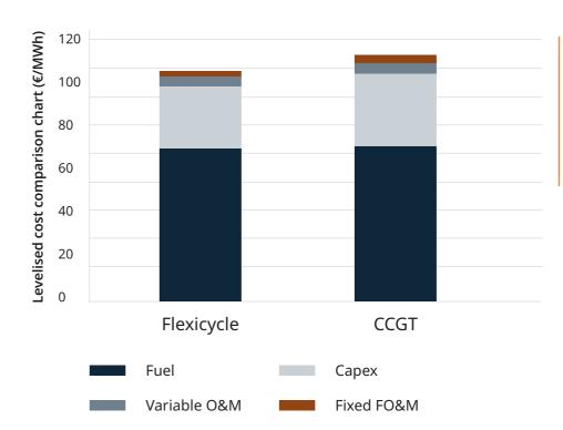
Levelised cost of electricity comparison on 6000 running hours & 100 annual starts. Wärtsilä Flexicycle is outperforming the CCGT plant in the intermediate operation. The higher onsite efficiency is resulting in lower fuel costs. Savings with Wärtsilä gas engine power plant 8 €/MWh, approximately 4.7 M€ per year.
