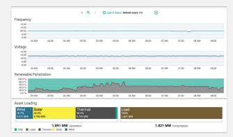
GEMS can monitor all assets within a system, such as Energy Contribution Monitoring. The GEMS dashboard shows data such as grid quality, renewable penetration, and asset loading.
