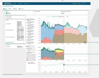
The GEMS dashboard illustrates monitoring and reporting capabilities: generation stack, Engine Dispatch Schedule, load and renewable forecasts. The GEMS user interface shown here gives insight into historic and forecasted asset loading via a stacked power plot.
