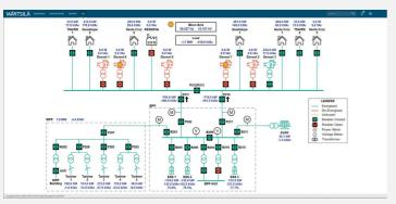
GEMS platform capabilities include 24/7 grid monitoring, including detailed single-line diagrams (SLDs).
