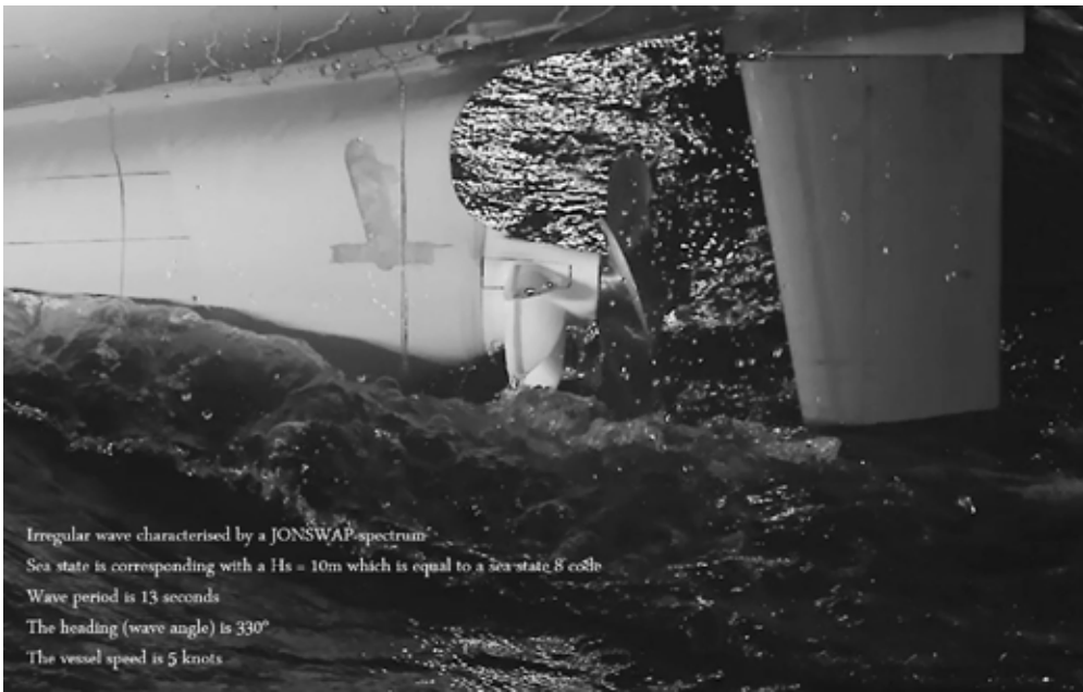
Model tests carried out for validating the strength of the EnergyFlow.
