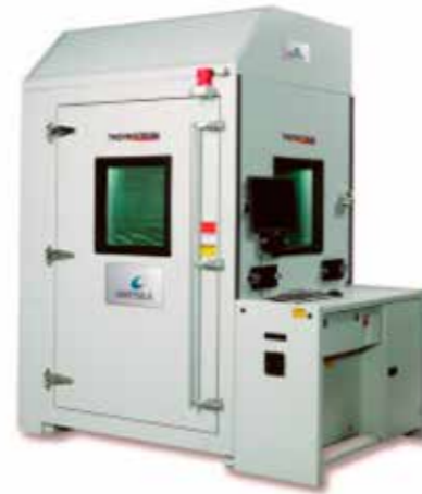
■ Fig. 4 - Accelerated ageing test - HALT.
