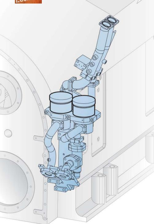
The fuel oil pulsation damper system mounted on a Wärtsilä 18V46 engine. Protective shields not shown in this illustration.
