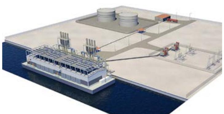
Fig. 13 – A typical power barge layout.
