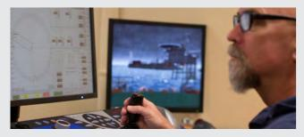
DP SIMULATOR allows for The Nautical Institute approved Dynamic Positioning training focused on operational procedures for adverse events, which are too complex and dangerous to train at sea
