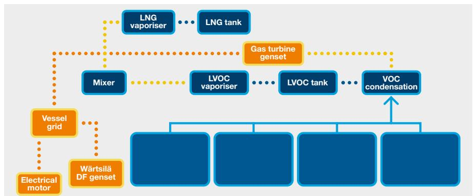
Emission transformed to fuel – 30-40% of fuel converted from waste
