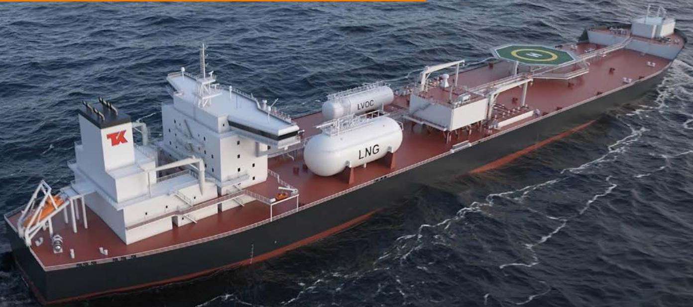
During offshore and onshore loading, storage and transportation of crude oil onboard vessels or in oil terminals, crude oil vapours, also known as volatile organic compounds (VOC), are emitted to the atmosphere. The emissions vary between 0.1 kg VOC per ton of cargo to 2.8 kg VOC per ton (offshore loading in bad weather). When liquified, this will be equal to hundreds of barrels of oil. The emissions are a substantial source of lost financial value and destructive environmental impact.
