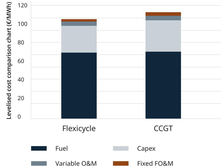
Levelised cost of electricity comparison on 6000 running hours & 100 annual starts. Wärtsilä Flexicycle is outperforming the CCGT plant in the intermediate operation. The higher on-site efficiency is resulting in lower fuel costs. Savings with Wärtsilä gas engine power plant 8 €/MWh, approximately 4.7 M€ per year.
