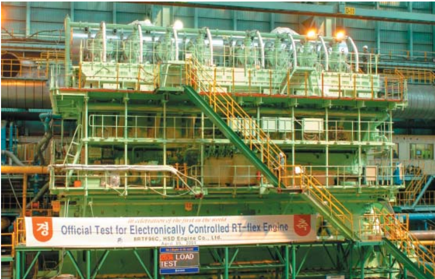
Fig. 18: The first Sulzer RT-flex96C common-rail engine: an 8RT-flex96C of 45,760 kW at 102 rev/min. [04#054]
