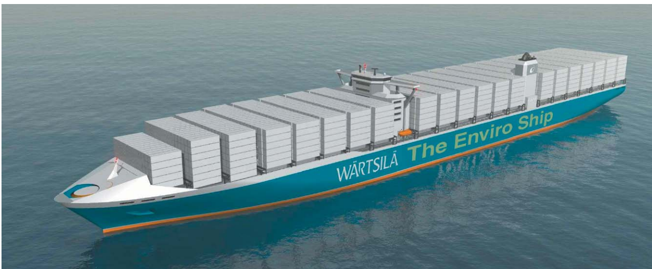
Fig. 19: The Enviro Ship concept can be illustrated by the case of a 10,000 TEU container liner powered by a Sulzer 14RT-flex96C common-rail engine with a Total Heat Recovery Plant. [04#052]
