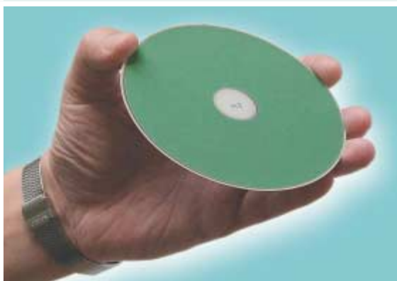
Fig. 3 Typical planar solid oxide fuel cells.
