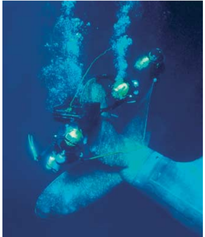
Underwater repair of propeller.
