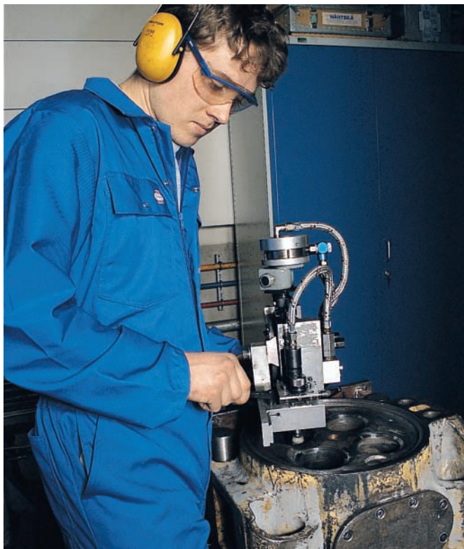
Machining of valve seats in cylinder head
