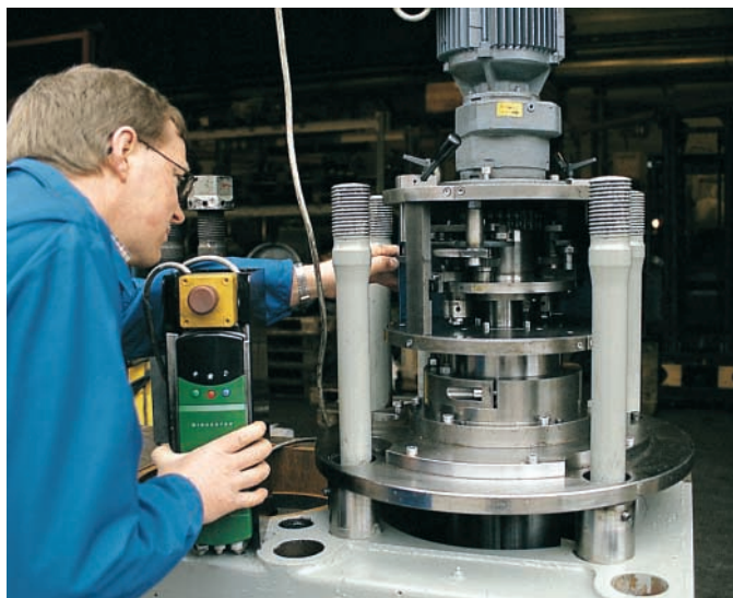
Machining of inner guides in cylinder block
