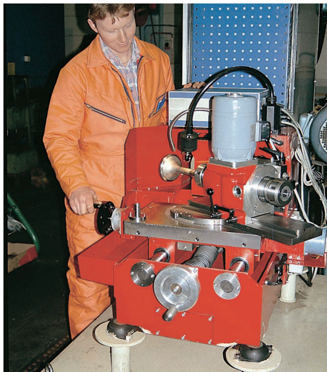
Grinding of valves
